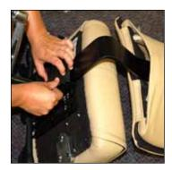
Tip the chair forward/over for clear access to the rear underside. Remove the plastic cover shielding the end of the back post for access to the bolts.
