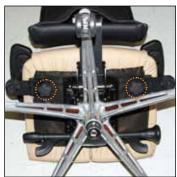
Activate seat height lever to maximum length, then tip the chair forward/over for access to arm brackets on underside of seat. If you're replacing both arms, do one at a time, noting the "slant" of the arms support may be mounted in two directions.
