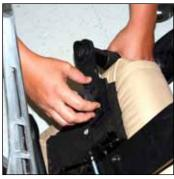
Set the armrest width as desired and firmly tighten the hand wheel.
