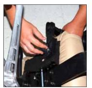
Locate where arms attach to underside of the seat. and remove the handwheel. Keep all washers in place for later reinstallation.
