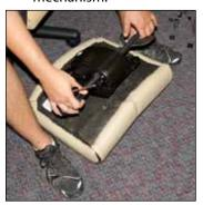
7. Position new mechanism on the seat in same manner as the old one, and center the holes for the screws over the same T-nut receptacles. Reinstall and tighten the screws being careful to not over-tighten them.
