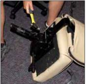
Hold the end of the cylinder with one hand, and hammer the mechanism around the cylinder entry point. \*\* Several strong blows may be required to dislodge the cylinder from mechanism.
