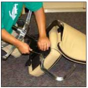
Position the new arm where the old arm was previously set, and replace the 3 Phillips head screws. Tighten in rotation.
