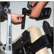
Slip the old arm support out and replace with the new arm. Replace the hand-wheel with washers (be careful not to crossthread).
