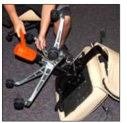
In the chair forward/over until the base is off the floor. Hold one leg of the base and strike the cylinder protruding through the base, using a plastic hammer. The force will dislodge the base.\*
