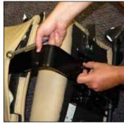
With the nuts removed, 3. hold the back support steady with one hand, and push the bolts up and out of the back post, allowing the back post to slide out.
