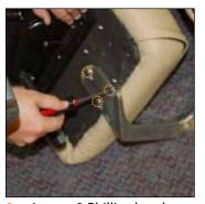
Locate 3 Phillips head screws that secure the arm to the underside of the seat, and remove all, setting aside for later reinstallation.
