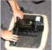
With all Phillips screws revealed, and removed, the mechanism can now be lifted off the seat
