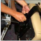
3 bolts, and gradually tighten each in rotation so all are equally set. Replace plastic cover (from Step 1).
